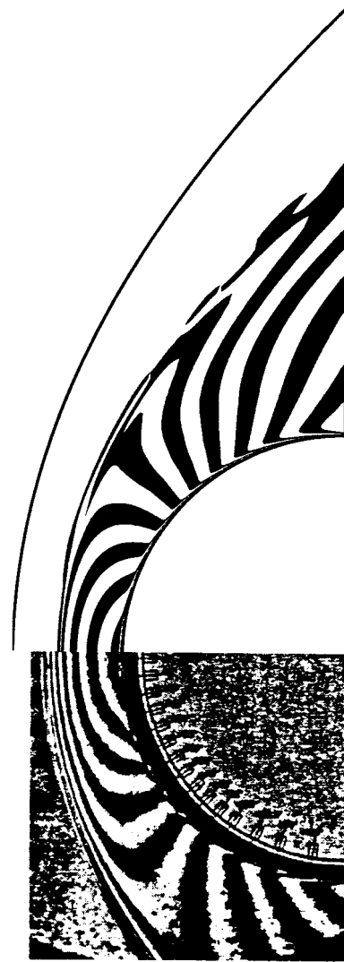
FIG. 8. Computed interferogram (top) compared with the experimental data of Sanderson (bottom).
