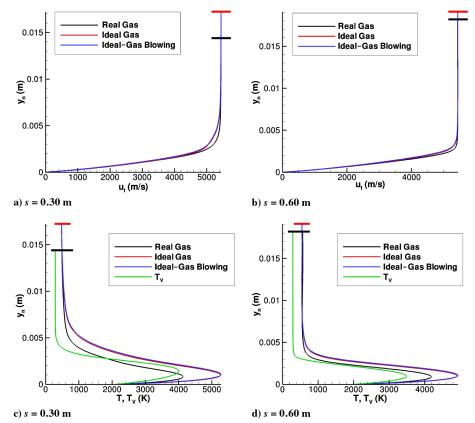
Fig. 16 Steady-state profile comparison between the three simulation cases for two streamwise locations. Shock heights are marked for clarity.
