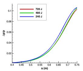
Fig. 11 Grid convergence study with three different grid densities in the wall-normal direction for the 525 kHz surface pressure perturbation.
