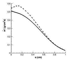
Fig. 7 Comparison of surface mass flux, where s is measured on the surface streamline and s = 0 corresponds to the stagnation point. The dashed line is from [4], and the solid line is from the current simulation.
