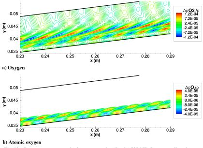
Fig. 22 Instantaneous perturbation contour plots for the 525 kHz frequency disturbance.
