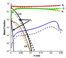
Fig. 9 Comparison of species mass fraction along the stagnation line to [6]. Dashed lines are from [6], and solid lines are from the current simulation.
