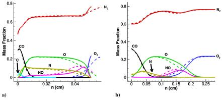
Fig. 3 Comparison of a) mass fractions on the stagnation line, and b) mass fractions at the sphere exit. Dashed lines are from [4], and solid lines are from the current simulation.
