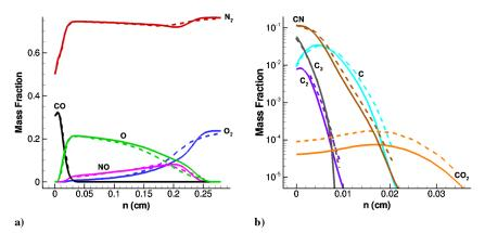
Fig. 6 Comparison of a) mass fractions at the sphere exit, and b) a close-up of the mass fractions at the sphere exit. Dashed lines are from [4], and solid lines are from the current simulation.
