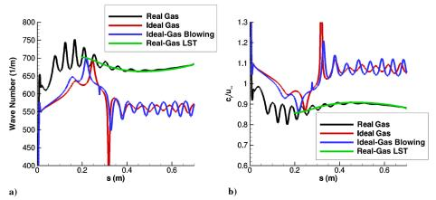
Fig. 20 Comparison of a) wave number, and b) phase velocity nondimensionalized by the freestream velocity for the 525 kHz disturbance.
