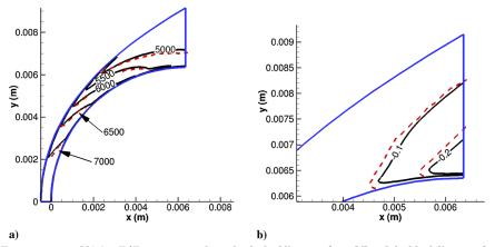
ig. 5 Comparison of a)  $T_V$  contours, and b)  $1 - T/T_V$  contours, where the dashed lines are from [4] and the black lines are from the current simulation.
