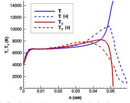
Fig. 1 Translation-rotation temperature and vibration temperature comparison on the stagnation line.
