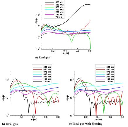
Fig. 23 Pressure perturbation amplitude at the wall computed by DNS.
