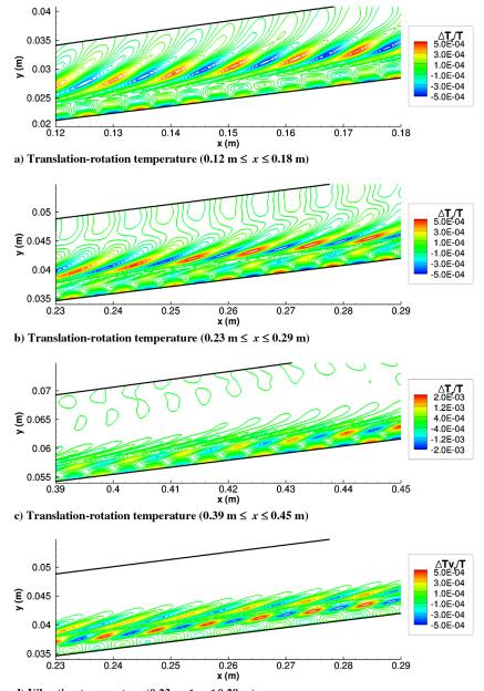
d) Vibration temperature (0.23 m  $\le x \le 0.29$  m) Fig. 21 Instantaneous perturbation contour plots for the 525 kHz frequency disturbance.
