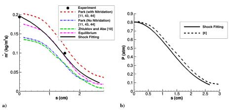
Fig. 8 Comparison of a) sphere surface mass blowing rates, and b) sphere surface pressure. Dashed lines are from [6], and solid lines are from current simulation.
